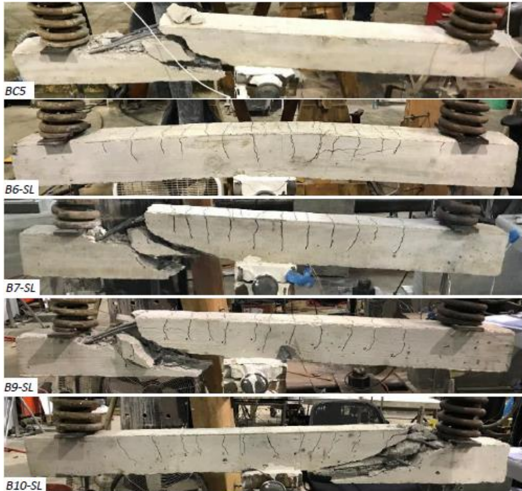
Figure 3-65. Beam series II failures.
