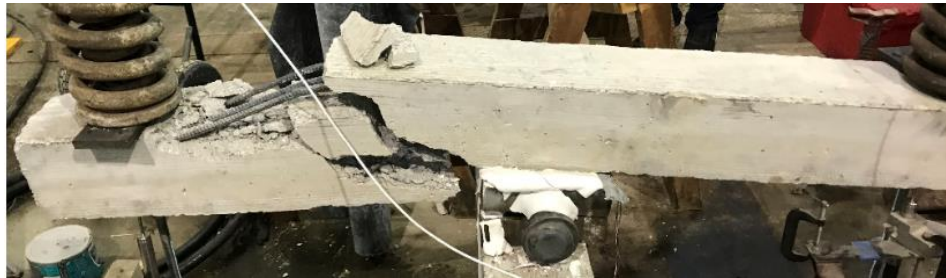
Figure 3-40. Beam 5 (BC5) failure.
