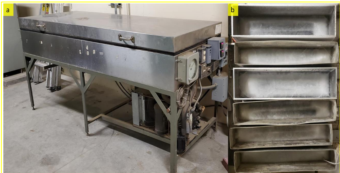
Figure 2.12 (a) Freeze-Thaw cycling test apparatus. (b) Samples under freezing conditions.
