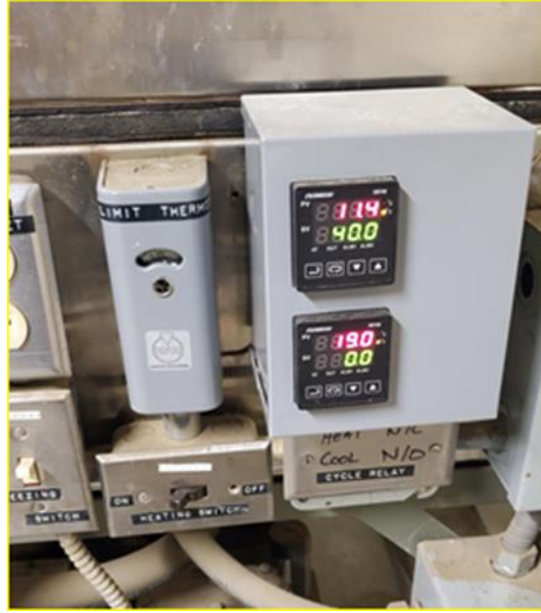
Figure 2.13 Freeze-thaw chamber temperature set range of 18°C to 4°C (0°F to 40°F)
