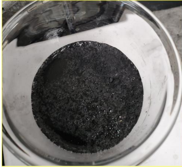
Figure 2.2 Al 2 O 3 /CNFs aqueous solutions showing excessive amount of air bubbles during mixing with superplasticizer.
