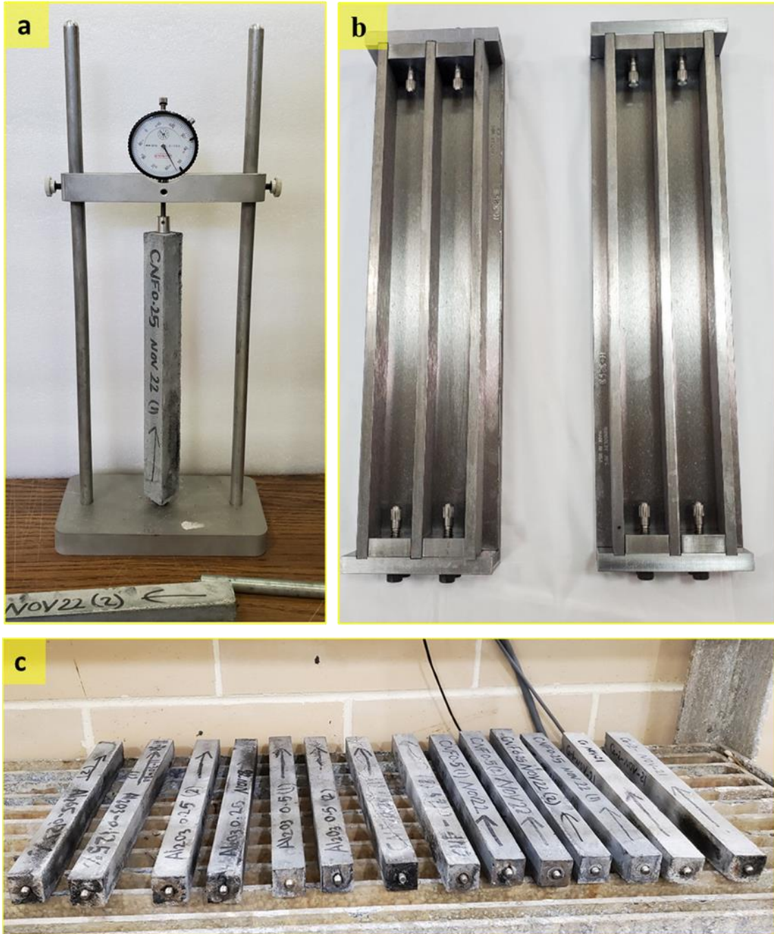
Figure 2.14 (a) Length comparator and dial gauge, (b) Steel prism molds of dimensions 1"×1"×10", 2-Gang. (c) Cement mortar prism samples in controlled-humidity room.
