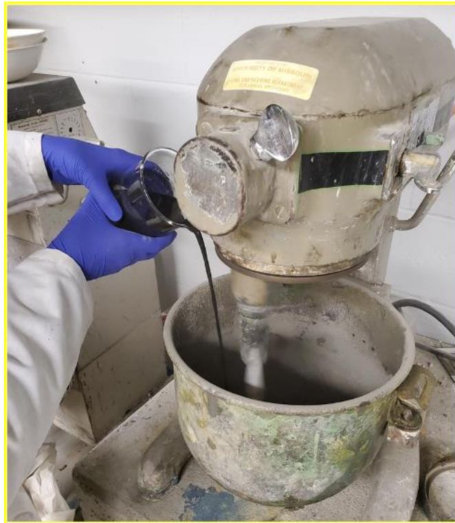
Figure 2.4 \text{Al}_2\text{O}_3/\text{CNFs} or CNFs suspension pouring during mixing with cement and sand.
