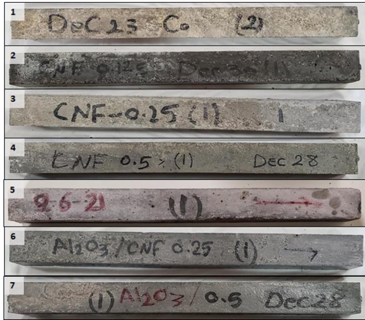
Figure 3.19 Samples after 50 freeze-thaw cycles, (1) C0, (2) CNFs-0.125%, (3) CNFs-0.25%, (4) Al 2 O 3 /CNFs-0.125%, (5) Al 2 O 3 /CNFs-0.25%, (6) Al 2 O 3 /CNFs-0.5%.
