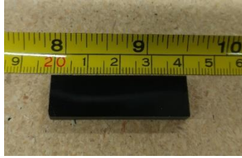
Figure 3.7: ILSS specimen dimension
