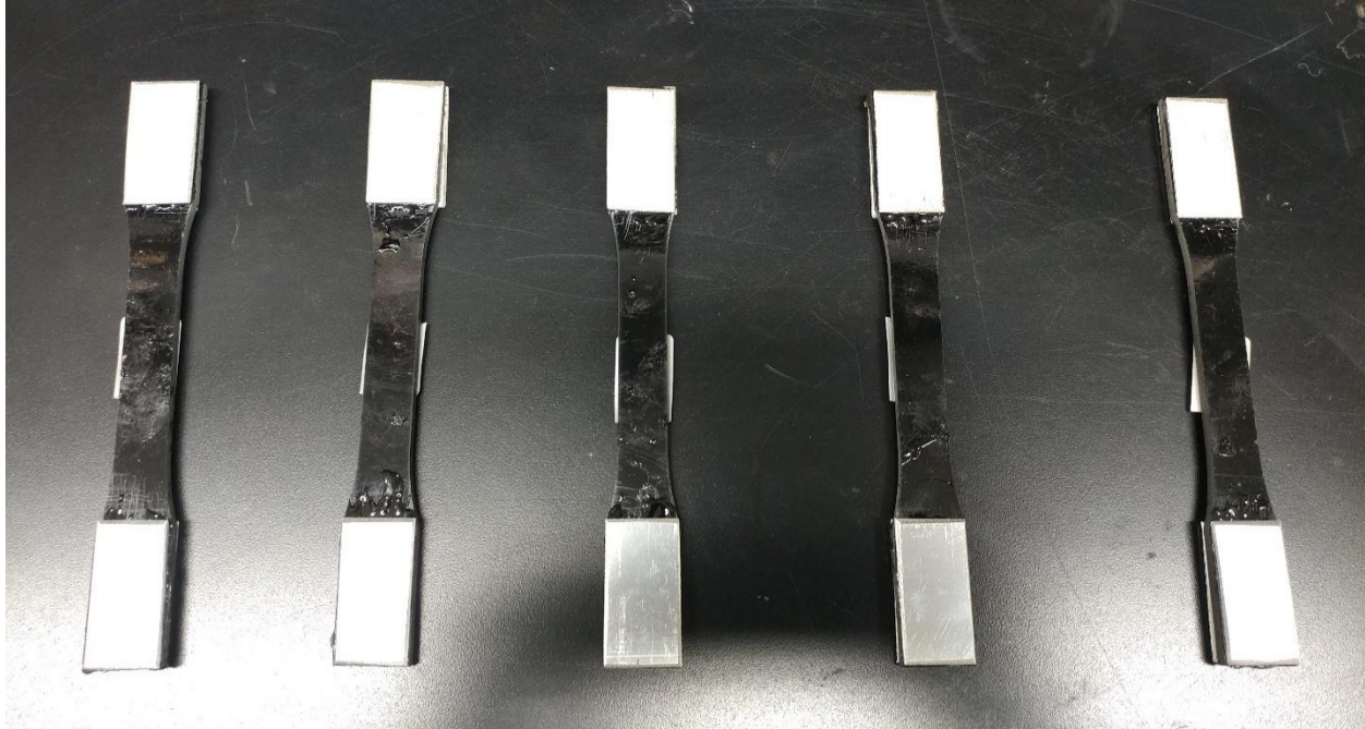
Figure 3.16: Dog – bone specimens which have been fabricated for the tension test in this experiment
