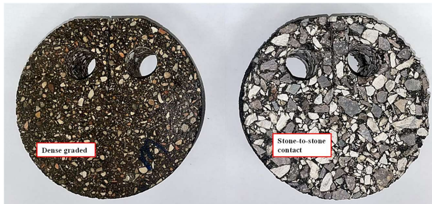
Figure 1.2 Lab specimens of dense graded versus SMA mixes
