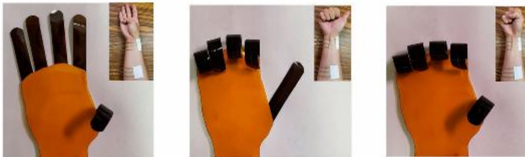
Figure 2.5.13 Photographs, indicating the control of a soft robotic hand via EMGs recording.
