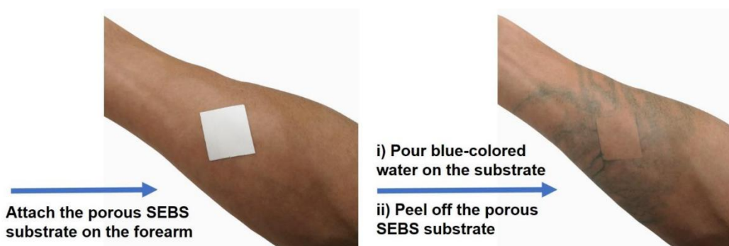
Figure 2.3.15 Waterproof test. A porous SEBS substrate was attached onto the forearm of a human volunteer. Then, the blue-colored water was poured onto the substrate. Water did not penetrate into the skin area covered by the porous SEBS substrate, indicating its outstanding waterproof capability, largely because of its high hydrophobicity and conformal contact with the skin.
