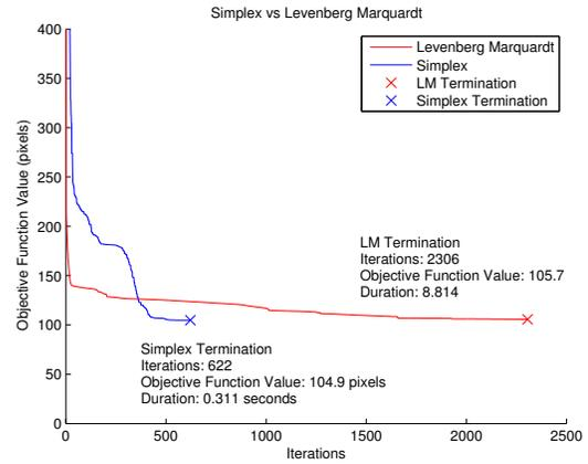
Fig. 2. Simplex algorithm vs. Levenberg-Marquardt
