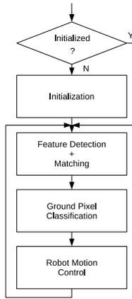
Fig. 3. Flowchart of the Target Follower Navigation Algorithm
