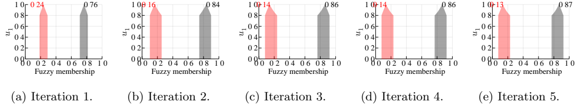
Figure 3.22: The vertical cut dampened LFCM membership functions u_{1,1} and u_{1,2} with m = 2 and \beta = 0.8 at different iterations. The black functions represent u_{1,1} , whereas the red functions represent u_{1,2} .
