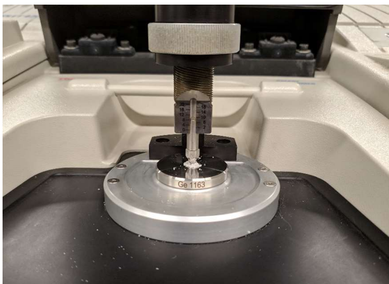
Figure 3-4: ATR-FTIR assembly with microplastic sample
