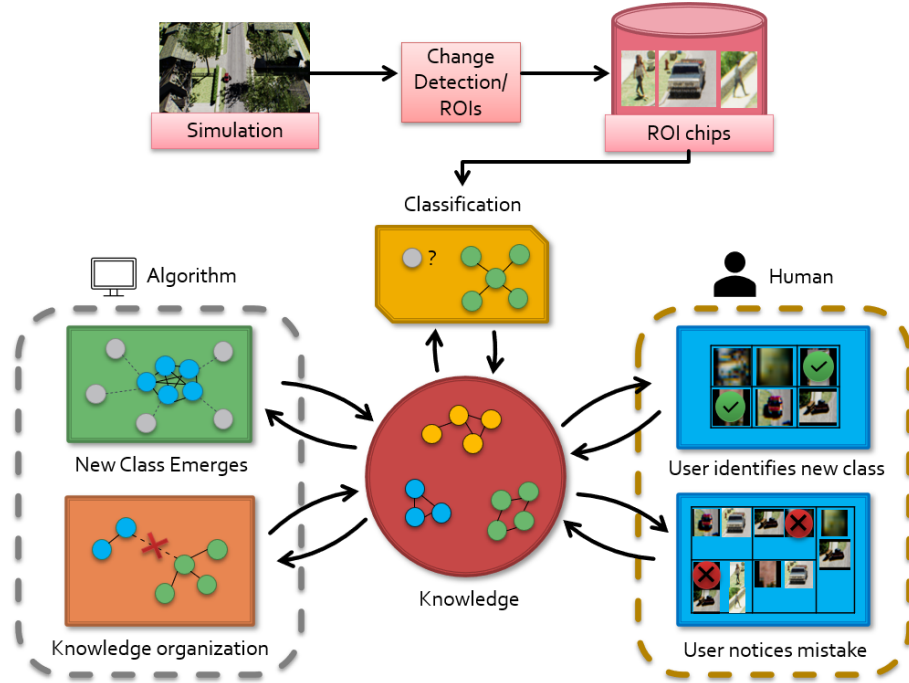
Figure 4.1: High-level overview of SSHING. In our aerial application, change detection is used to identify regions of interest in imagery. SSHING attempts to classify ROIs based on machine learned DNN features. SSHING operates in a self-supervised fashion to identify new classes and evolve its knowledge. SSHING also makes use of a human-in-the-loop to accelerate learning, refine its knowledge, and/or answer questions it cannot otherwise solve.
