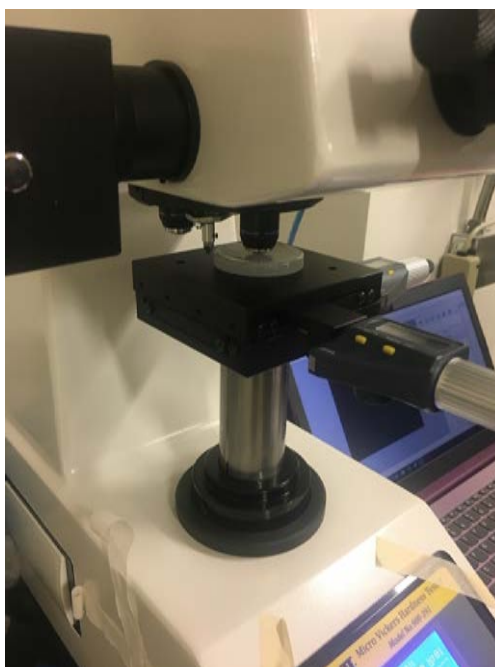
Figure 17: Micro-Vickers Testing with SU-2100 coated polycarbonate.
