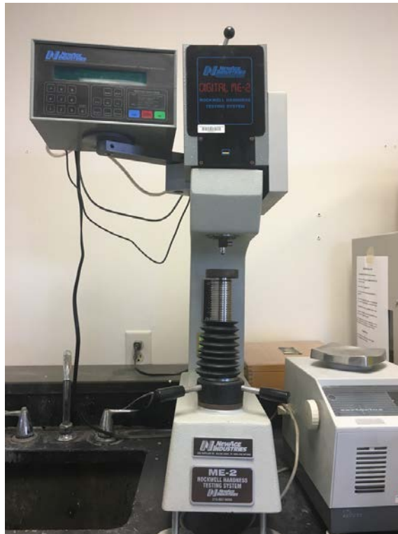
Figure 16: Rockwell Hardness measuring devices in the lab.
