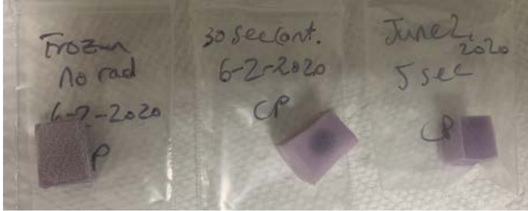
Figure 20: High flux Pink samples, L to R, frozen (no irradiation, frost seen), 30 second irradiation (swelling and discoloration seen), 5 second irradiation.
