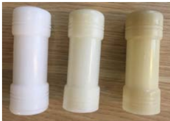
Figure 22: Pneumatic Tube Vehicles through progressive usage (new white tube at left).
