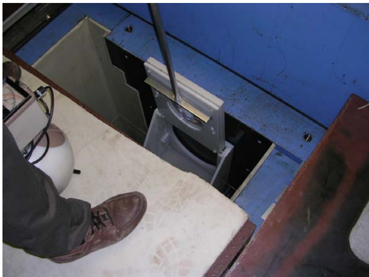
Figure 27: Inserting specimen into beamport position.
