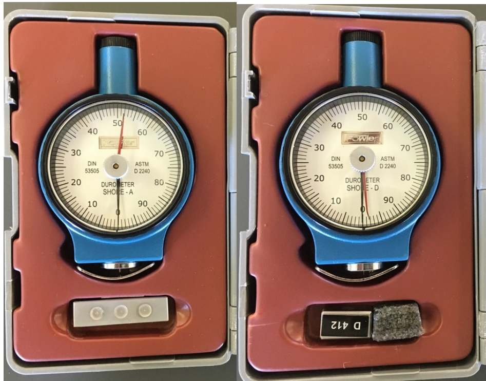
Figure 18: Shore A (left) and Shore D (right) Durometers.
