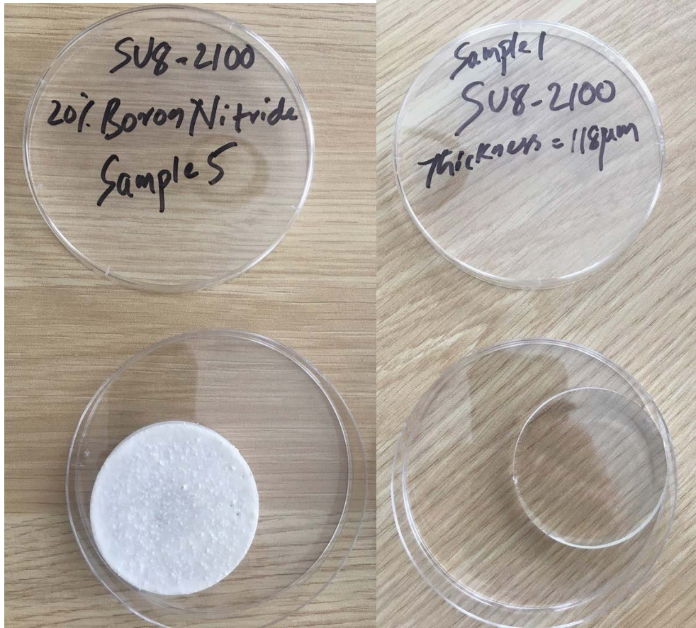
Figure 33: : Custom borated SU8-2100 Specimen with high boron nitride content and no boron nitride.
