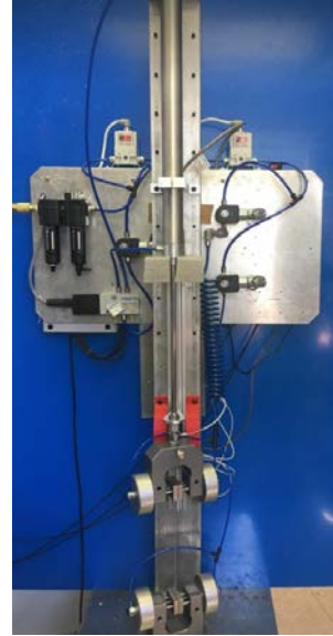
b) Pneumatic Testing Frame
