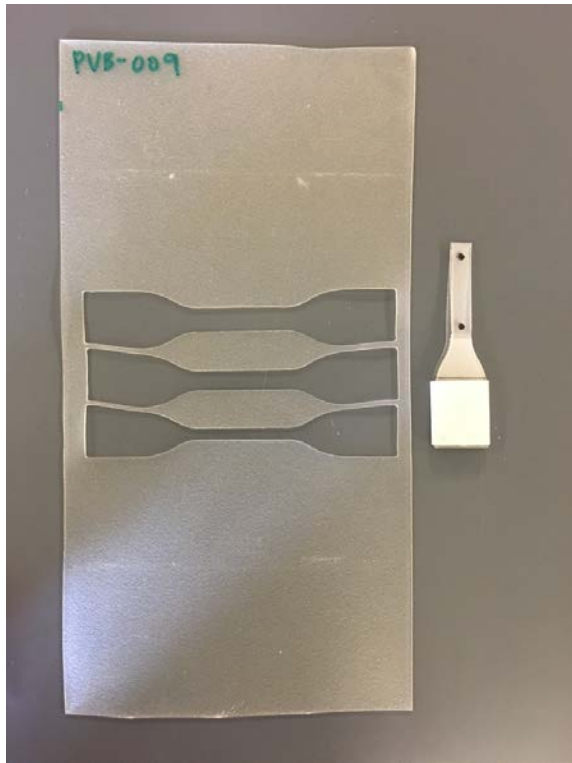
Figure 10: Static tensile specimen cut out from treated interlayer.
