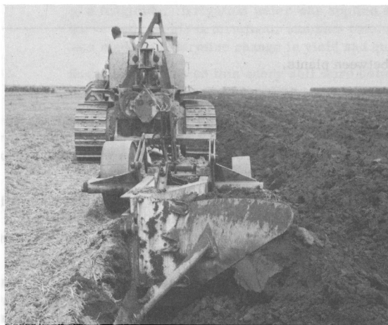
Breaking loam soil 27 inches deep at the Delta Center near Portageville, Missouri
