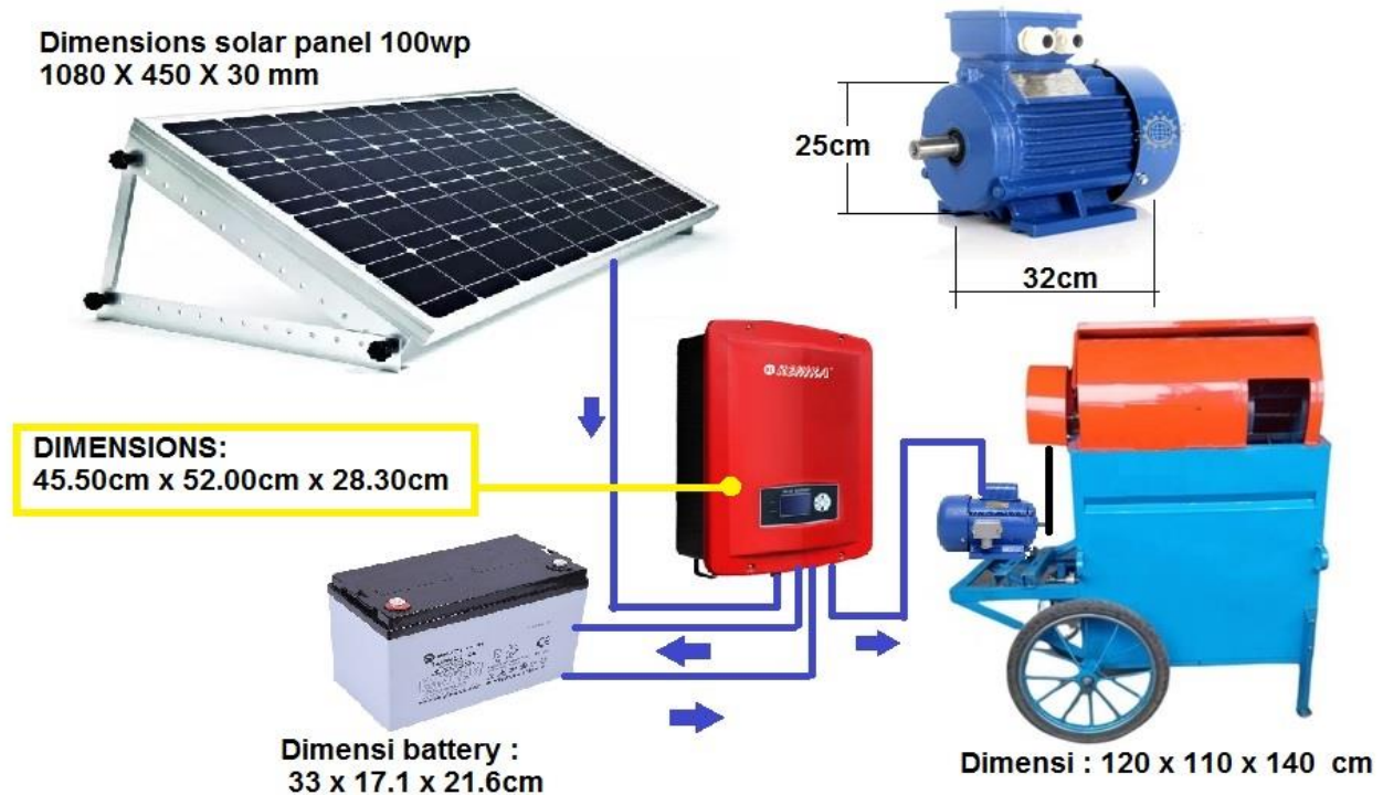
Figure 6. Rice milling SOLAR energy, Agricultural Technology Renewable Energy
