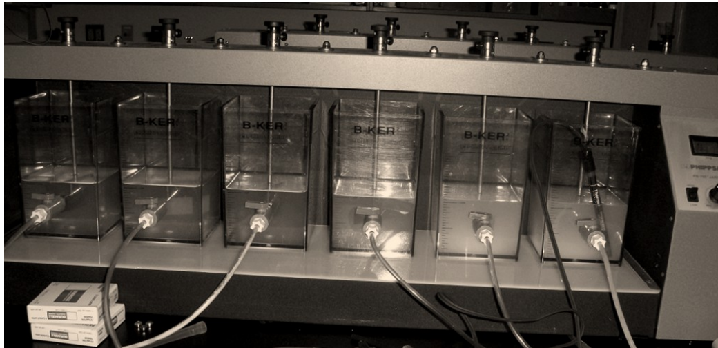
Figure 2-1: Jar Tester Apparatus
