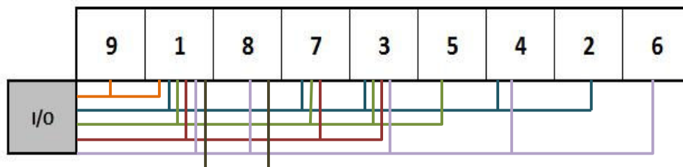
Figure 3.9 Item storage assignment after placing SKU 8 and SKU 9 close to the I/O location
