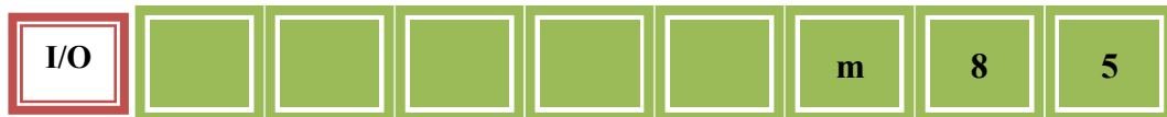
Figure 4.3 Linear permutation with unassigned item (i.e. represented as blank), assigned items (i.e. represented with a number inside) and the current worst available location (i.e. marked by "m")
