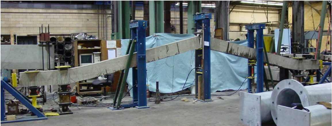
Figure 2-18. Photo of test PM-2 under catenary action
