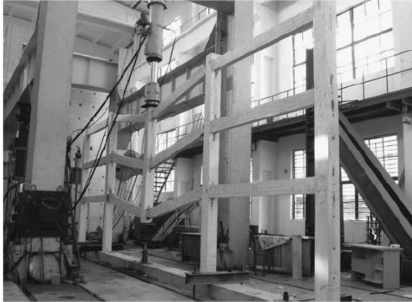
Figure 2-19. The tested four-bay and three-story one-third scale model representing a segment of a larger planar frame structure (Kunnanth, 2008).
