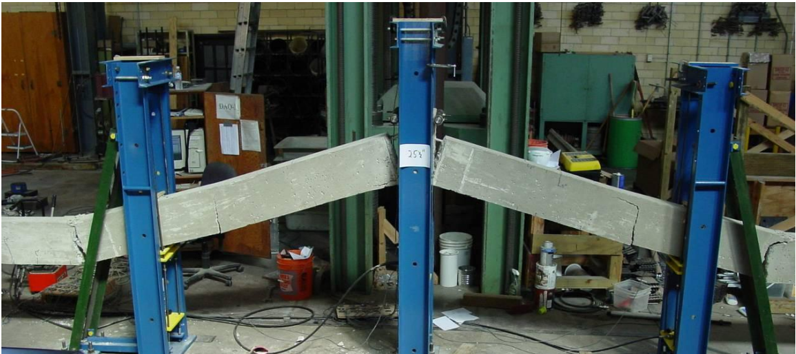
Figure 2-16. Photo of test NR-2 under catenary action
