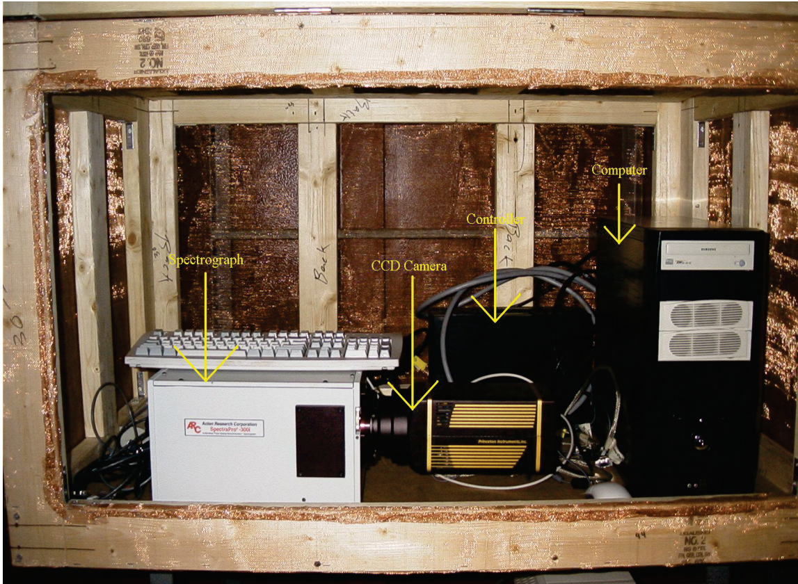
Figure 4.8 This photograph shows the location of the OMA diagnostic inside the shielded screen box. The screen box prevents MUTTS electromagnetic noise from interfering with OMA signal quality.
