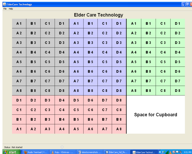
Figure 4-12: The Sensor display program when no sensor was activated. The letters A1-A8, B1-B8, C1-C8 and D1-D8 represent the 32 sensors on each installation system. Also the 4 installation systems are visually differentiated using different colors and thick line divider. (2)
