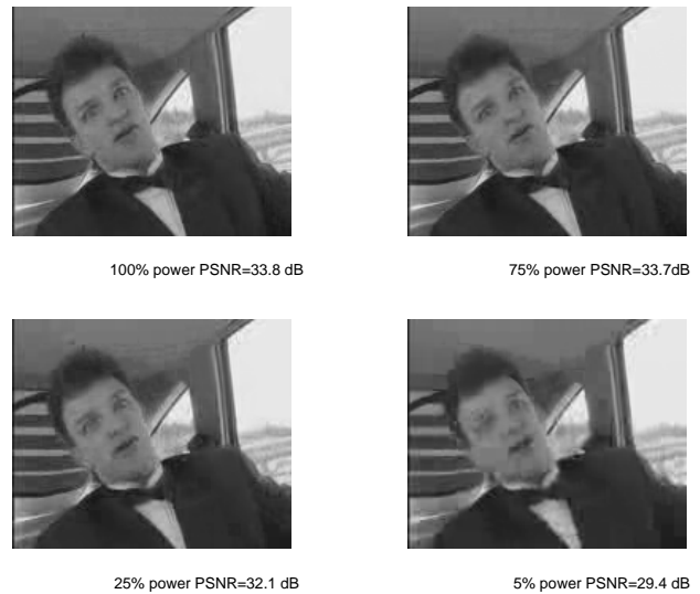
Fig. 13. The encoded "Carphone" QCIF sequence at 64 kbps and 15 fps for different power supply level.
