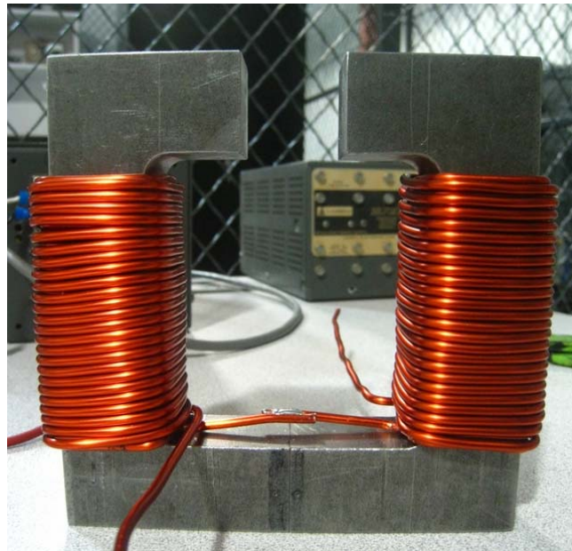
Figure 4.8: Magnetic core with 50 turns of 10 AWG magnetic wires at each side
