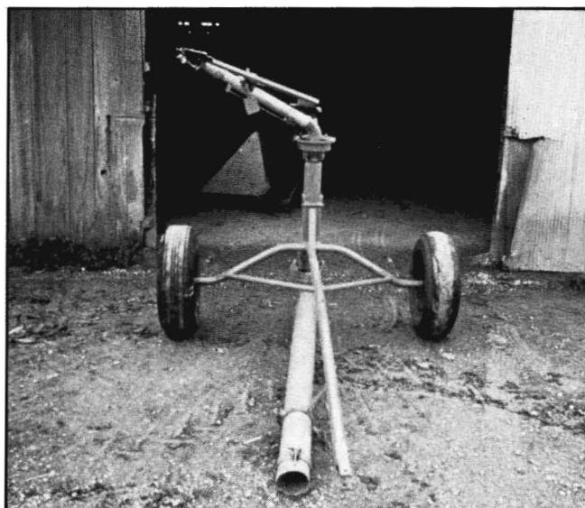
Figure 6. Some stationary big guns are mounted on wheels to make moving easier.
