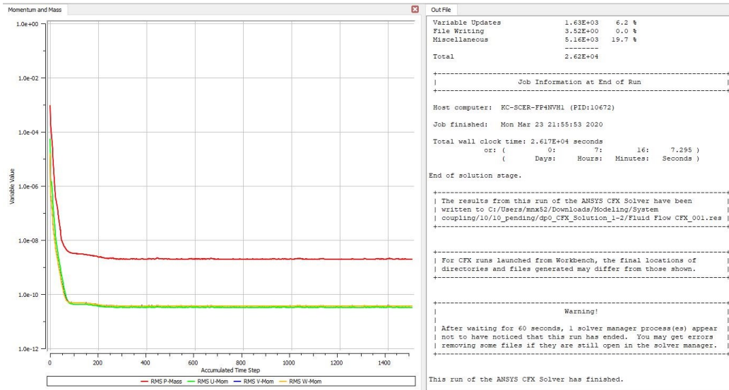
Figure 31: Mass and momentum residuals drops after solution convergence
