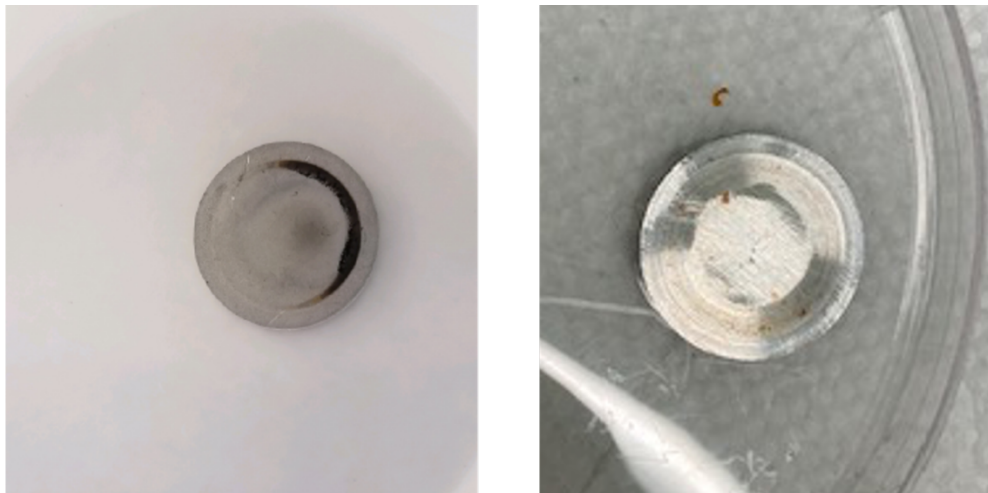
Figure 23: Left, photograph of previous aluminum capsule design after a 2 h irradiation at 20 \mu\text{A} . Right, photograph of new aluminum capsule design after a 2 h irradiation at 20
