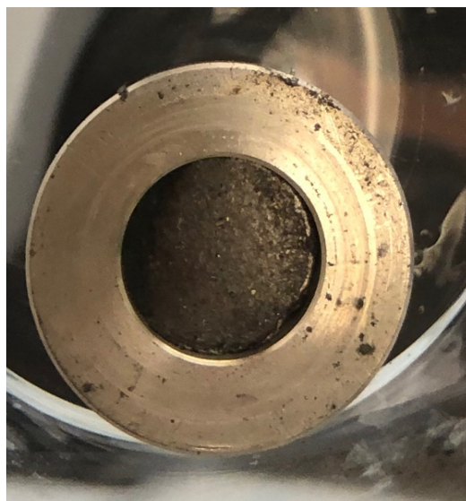
Figure 30: Photograph of the target after irradiation showing no discernable physical damage to the top graphite layer
