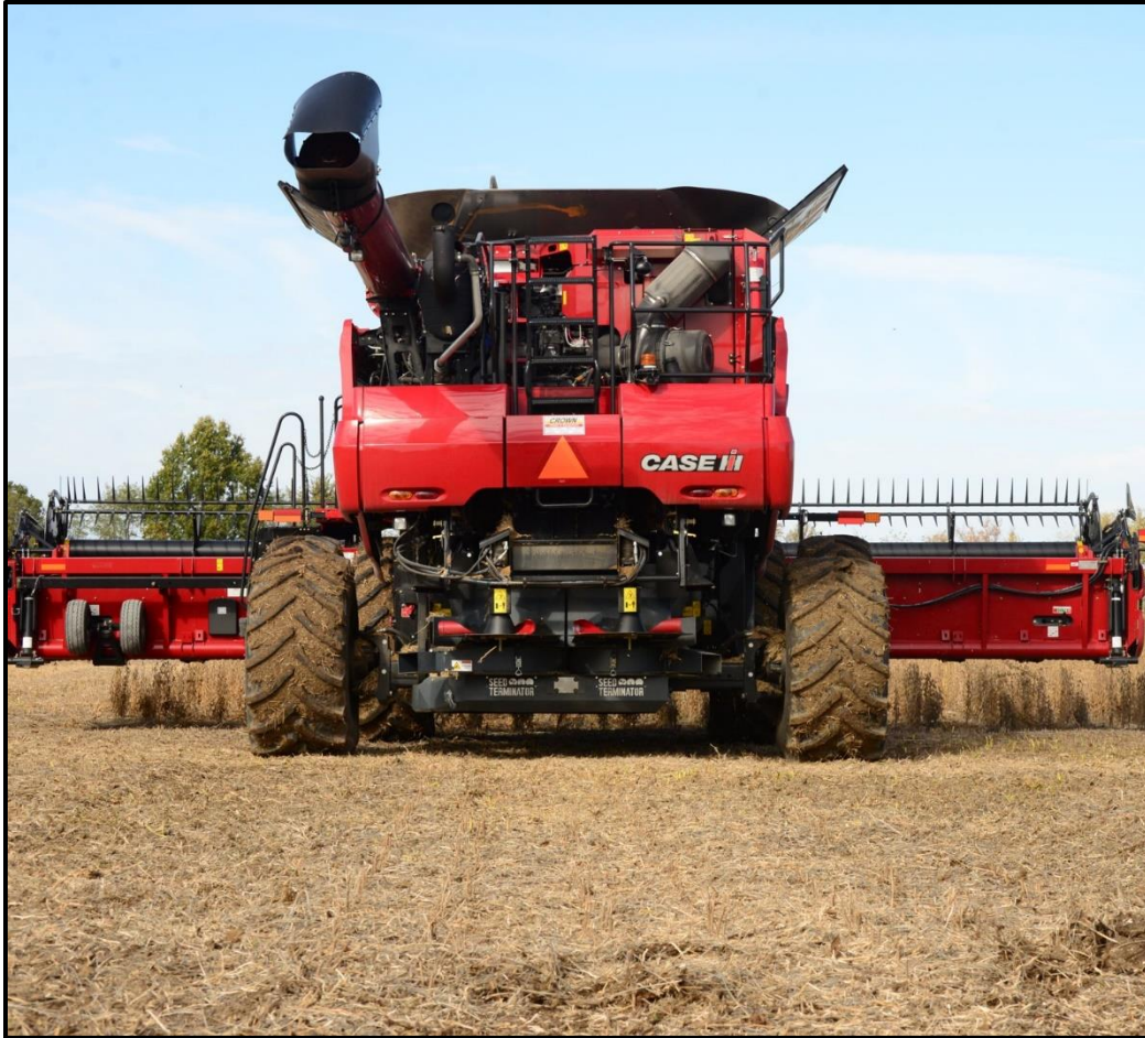
Figure 2.5. A Case IH 8250, equipped with a Seed Terminator™ implement.
