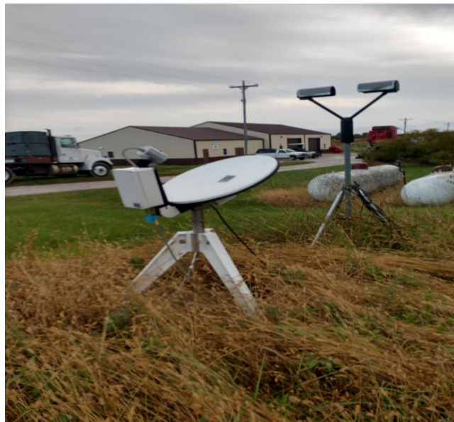
Figure 5 - The instruments used in this study. Located at Bradford Research Farm in Columbia, Missouri, the instrument on the left is the Micro Rain Radar, and the instrument on the right is the OTT Parsivel 2 laser disdrometer.
