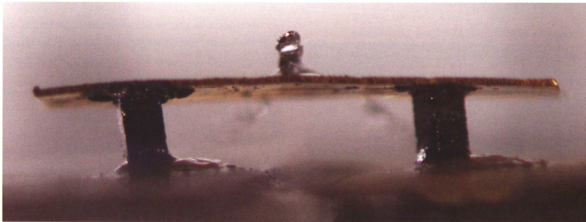
At left, mechanical engineering Assistant Professor, Gary Solbrekken and Graduate Assistant William Zhao, share a laugh in the lab where they are evaluating the intracellular phase change in single cells during cryopreservation. Above, the .75 millimeter by .5 millimeter “bridge” that controls the temperature when testing biological samples. When an electric current is applied to either of the towers that hold up the bridge, heating or cooling results where the towers meet the bridge.
