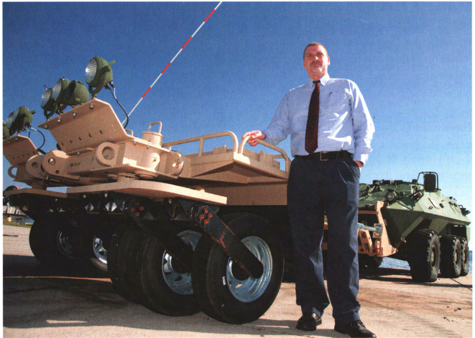
Alan Canfield poses in front of the Panama City Mine Roller, designed and built by his team at the Naval Surface Warfare Center in Panama City. The equipment is credited with saving the lives of many soldiers by protecting them from improvised explosive devices – IEDs.
