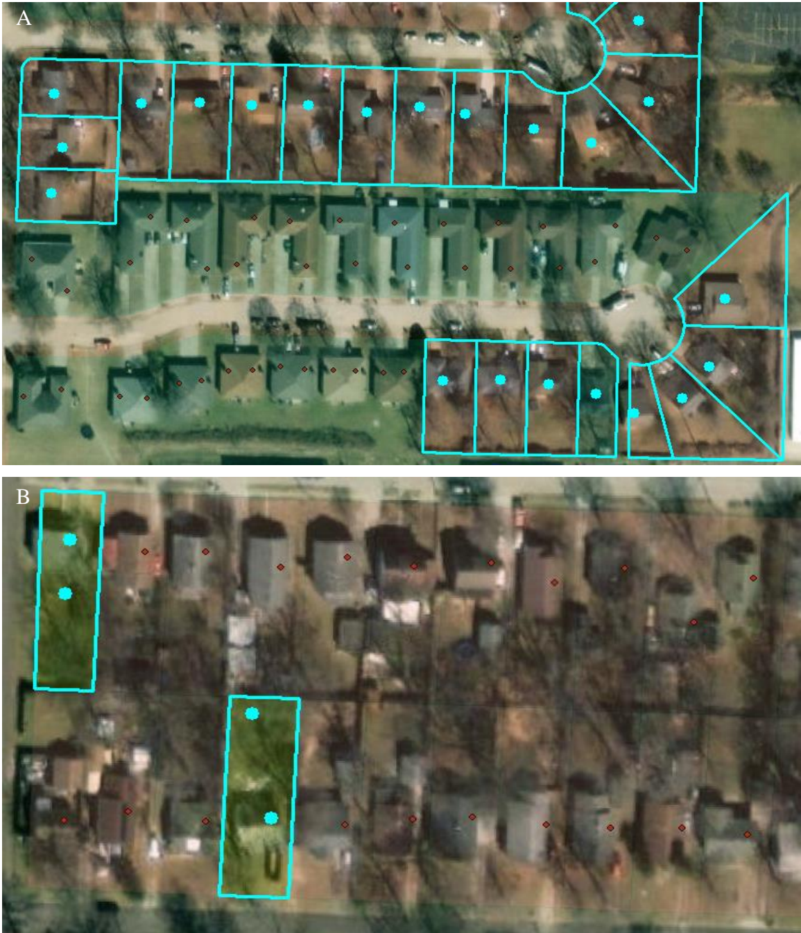
Figure 3. 2 Manual verification process of each polygon is linked to only one address point for single-family residential land. (A) the identification of appropriate polygons, (B) identified single-family residential polygons (represented by red colors), misidentification (represented by green colors)
