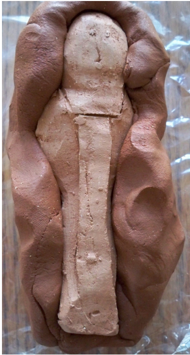
Figure 43. Impressing a completed figurine To form a new mold
