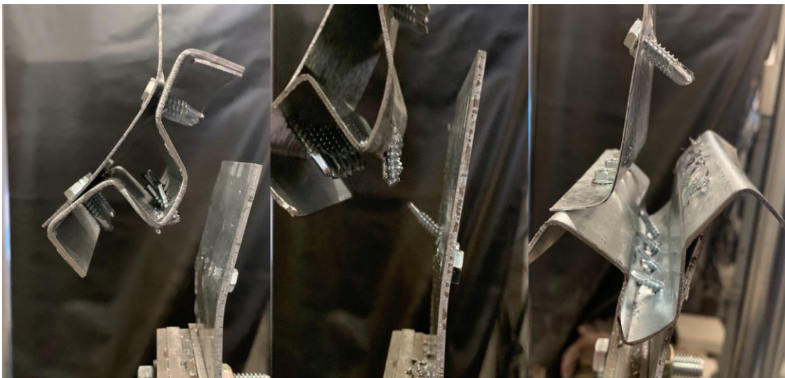
Figure 72: End Bearing USW Failure Types
