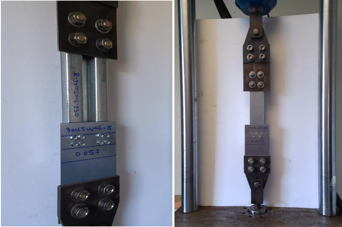
Figure 38: Aiges Connection Test Setup Pictures
