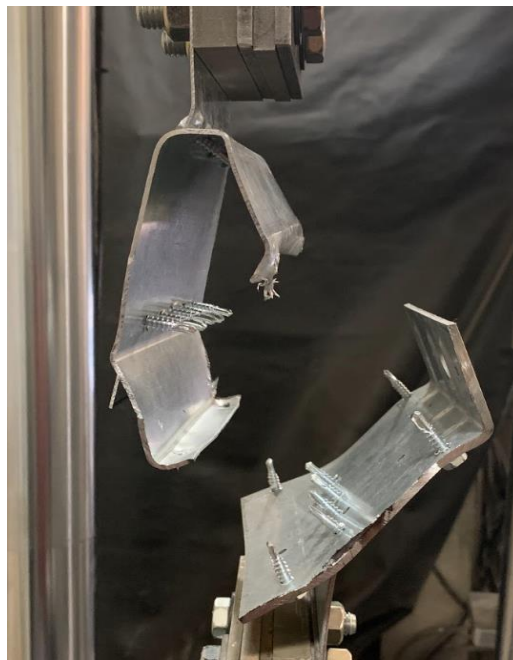
Figure 73: USWD End Bearing Failure
