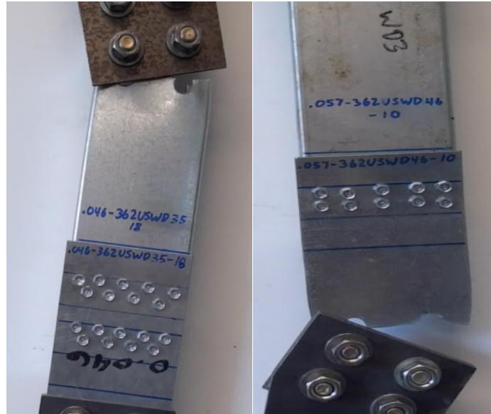
Figure 46: Bolt Hole Failure
