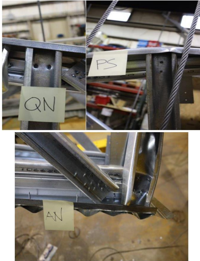
Figure 11: AG36-D35 Connection Failures – Treece [1]
