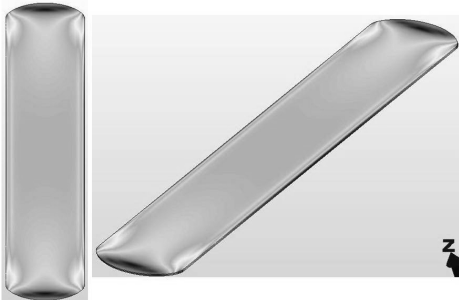
Figure 70. Partially constrained Von Mises stress gradient
