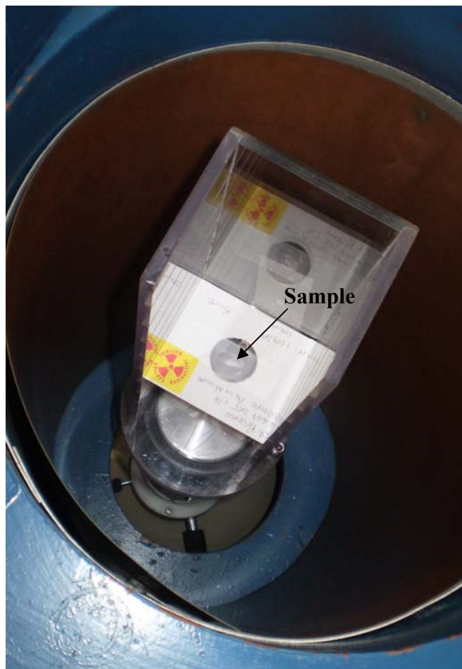
Fig. 2.9(b) A photograph of a fixed card-source holder on the REAR4 HPGe setup
