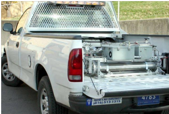
Figure 2.3.2 Kansas City fleet vehicle (left) using carbon monoliths produced from waste corncob as ANG storage.
