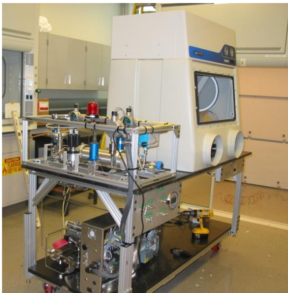
Figure 7.2.1. New room temperature manometric supercritical hydrogen sorption apparatus.
