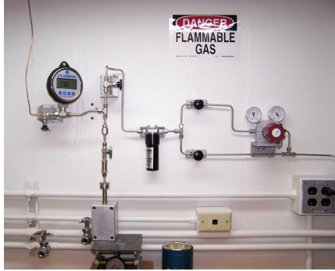
Figure 4.5.1. Left: Cartoon model of the rapid-screening hydrogen sorption apparatus. Right: Picture of the rapid-screening hydrogen sorption apparatus.
