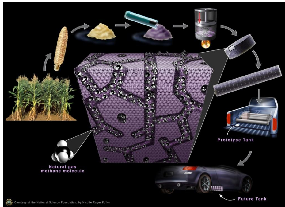
Figure 2.3.1 Overview of methane project with depiction of carbon manufacture process starting with waste corncob. Image Courtesy of the National Science Foundation, by Nicole Rager Fuller.
