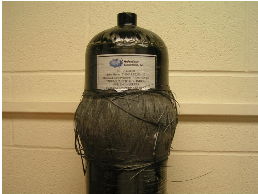
Figure 3-9. Image of T1000/epoxy burst COPV.
