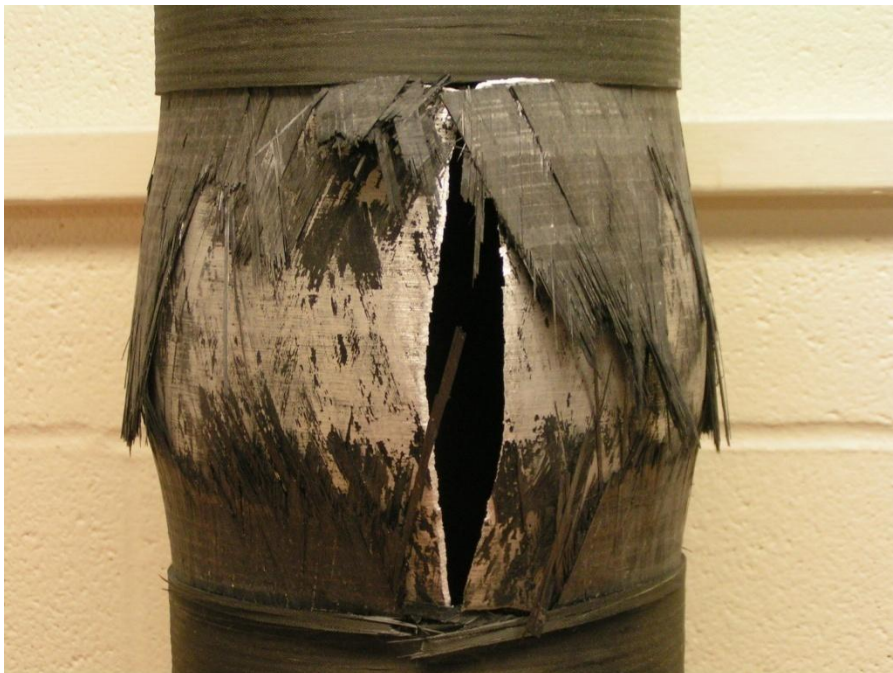
Figure 3-11. Zoom-in image of burst tank with IM7/epoxy with peel-ply treatment on the outer surface.
