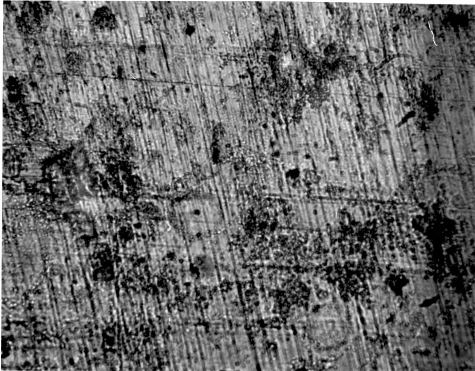
Figure 12. Dispersalloy Creep Specimen Photomicrographs (160X)
