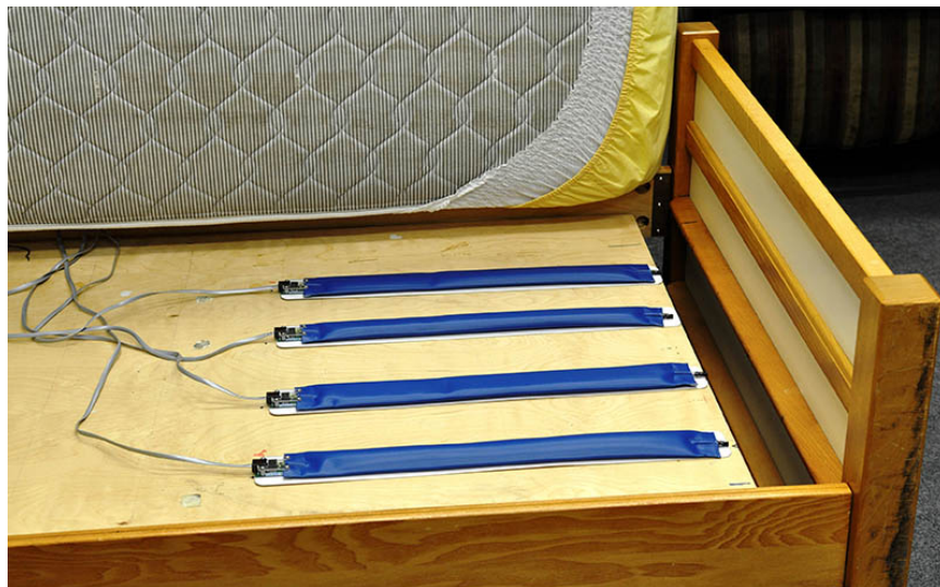
Figure 2.2: Hydraulic bed sensors monitor cardiovascular activity during sleep. Pressure-sensitive hydraulic transducers capture bio-physiological changes in bed
